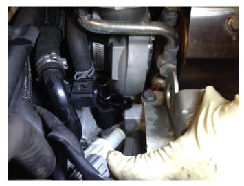
17. Use a small pick and disconnect the wiring harness from the bracket that is attached to the passenger side strut tower.
