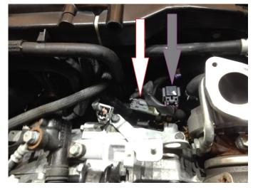
8. Disconnect the PCV valve from the hose leading to the crank case by using a narrow flathead screw driver. Slide it into the clamp and twist until the clamp breaks free.
