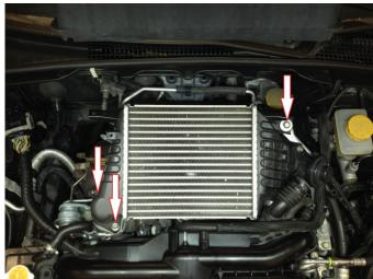
6. Loosen the hose clamp securing the intercooler to the throttle body by using an 8mm socket or flathead screw driver.
