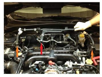
15. Working from the front of the intake manifold, the breather assembly connects to the turbo inlet line as seen in the image to the right. Loosen the hose clamp and pry the hose off the fitting. Once the breather assembly is free, cap the port with the provided 5/8" vinyl cap and secure with a zip tie (shown).
