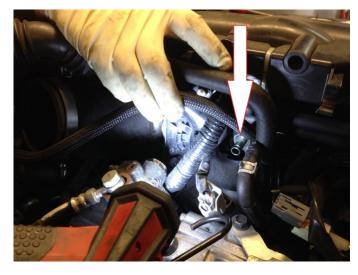
11. Located next to the turbo is the crank case drain port. To remove the pre-existing hose fitting attachment simply pull up on the hose until it pulls from the port on the engine block.
