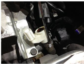
9. Once the PCV is free, use the provided ½" vinyl cap to cover the port. Secure it with a zip tie. You may then reinstall this into the original connector it came out of and set it aside.
