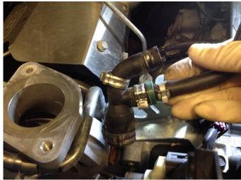
12. Remove the forward most valve cover breather hose on each valve cover. These hoses connect through a plastic crossover pipe that will be removed next.
